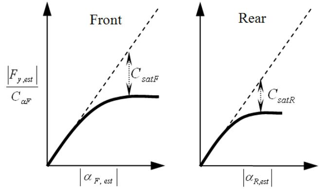
Fig. 3. Axle Force Saturation for Under Steering Vehicle
