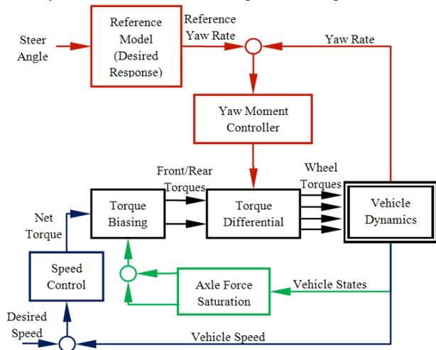
Fig. 4. Schematic of Stability Control Architecture
